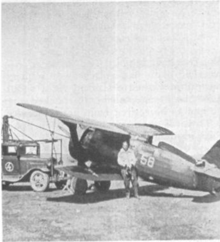
The Russian fighters' powerful engines had to be started by the above device.
