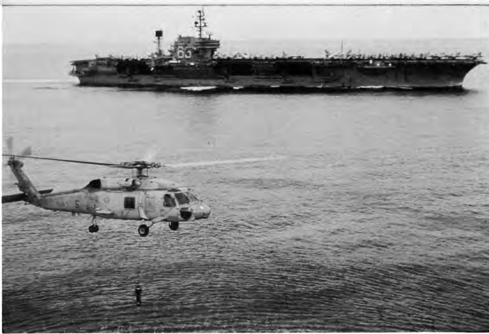
The SH-60F differs from the earlier SH-60B primarily in the mission equipment installed. The SH-60F replaces the search radar, sonobouys and MAD gear with a dipping sonar and enhanced ASW avionics. This SH-60F Ocean Hawk is assigned to HS-4 aboard the USS KITTY HAWK (CV-63). (Sikorsky)
