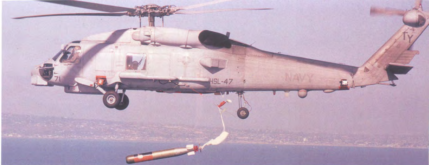
(Below) The Honeywell and Gould Mk 46 Mod 5 torpedo is the current standard aircraft and surface launched torpedo in the US Navy. This torpedo weighs 507.1 pounds (230 kg), including a 97 pound (44 kg) warhead. (Dann)
