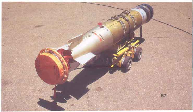
(Below) The SH-60B/F can carry up to three Mk 46 Mod 5 torpedoes, two on the port side and one on the starboard side. The Mk 46 is an acoustic homing torpedo with counter-rotating screws. The orange object at the rear of the torpedo is a parachute, which both slows and aligns the weapon prior to water entry. (Dann)
