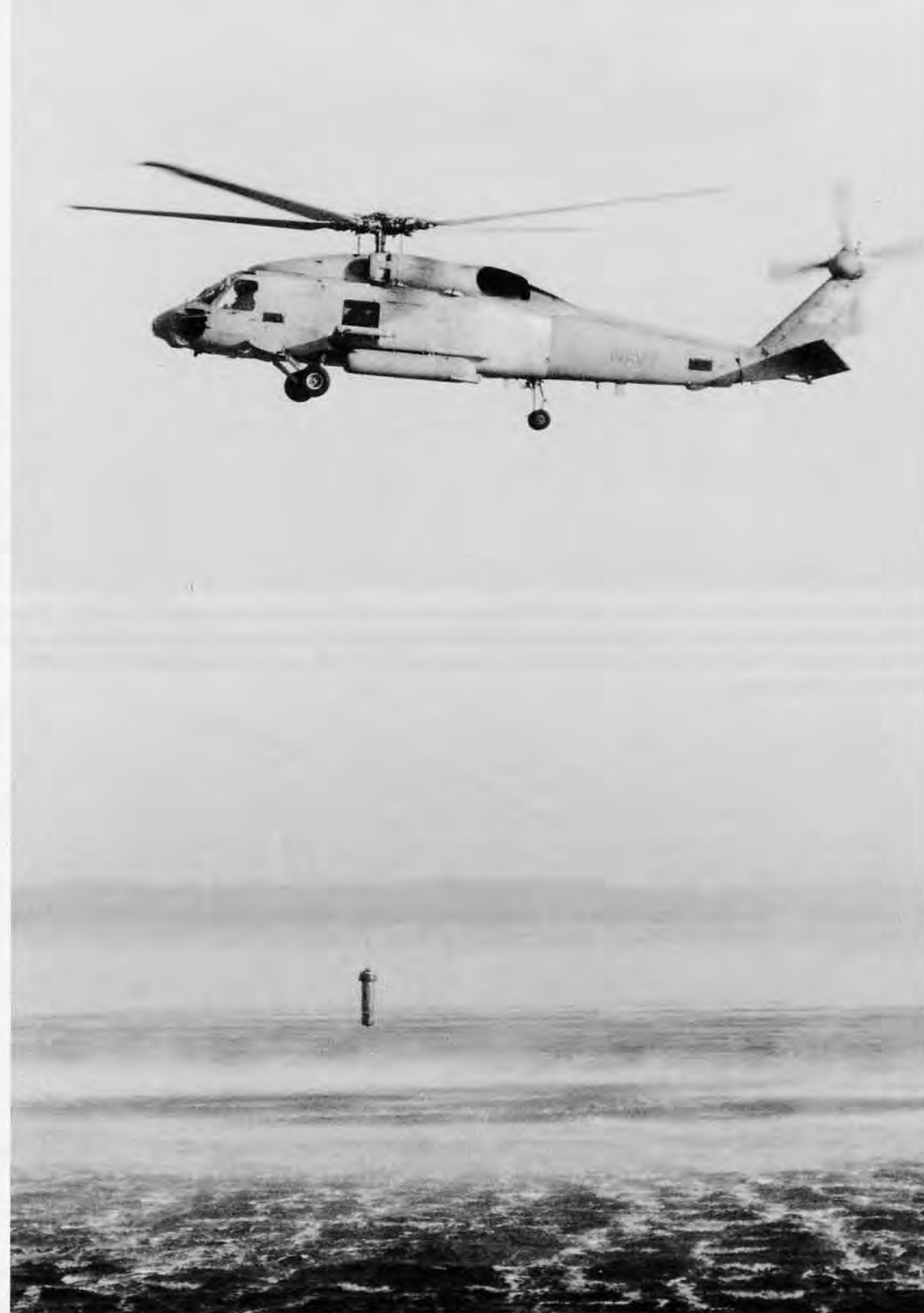
The SH-60F Ocean Hawk (CV Helo) is the Navy's new inner-zone anti-submarine warfare helicopter, replacing the SH-3 Sea King. This Ocean Hawk is lowering its Bendix active dipping sonar to begin a sonar sweep of the surrounding area. (Sikorsky)
