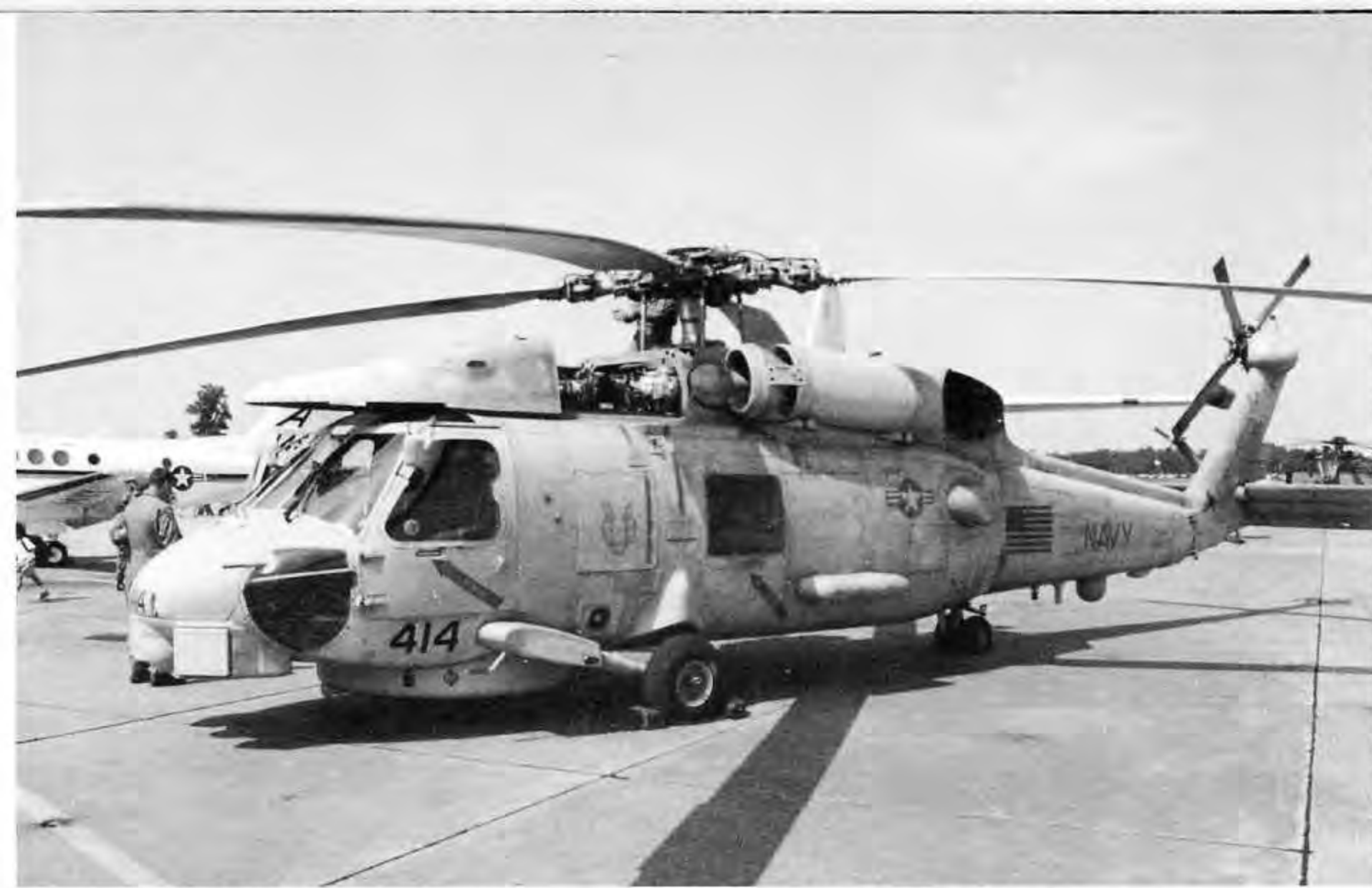
This HS-60B of HSL-40 parked on the ramp at NAS Mayport, Florida has the forward sliding fuselage fairing opened revealing the flight control system, hydraulic pumps and other engine accessories. (Author)
