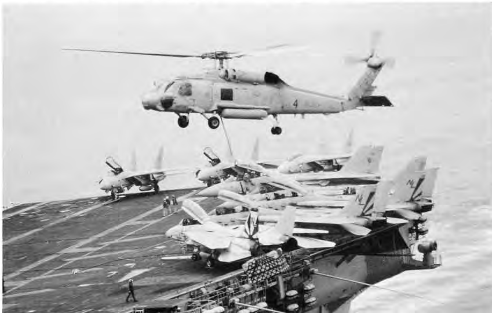
This SH-60F of HS-4 aboard USS KITTY HAWK is bringing in a sling load of supplies. Vertical Replenishment (VERTREP) is an important secondary mission for the SH-60F. (Sikorsky)
