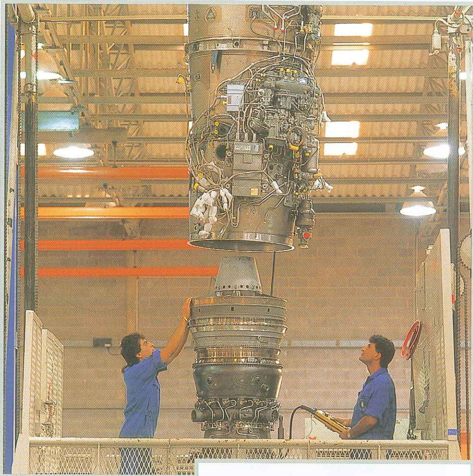
PWA - F100 final assembly line
